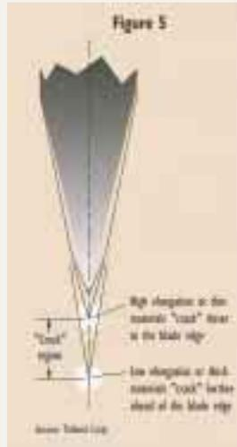
**Figure 5:** Razor slitting is, in essence, the creation of a "controlled crack" immediately ahead of the blade edge. The mechanical properties of the material and the shape of the edge determine how and where this crack forms. If the crack forms close to the edge, the process is relatively stable. If the crack forms far ahead of the tip, the process may become unstable.
