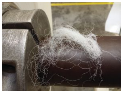
FIGURE 7. Angel hair from improper overspeed
