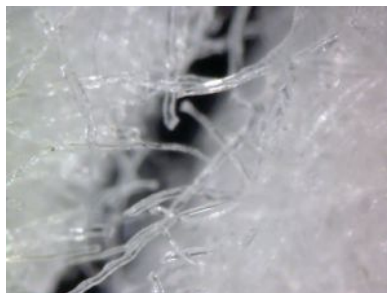
FIGURE 8. Microfiber structure of non-wovens
